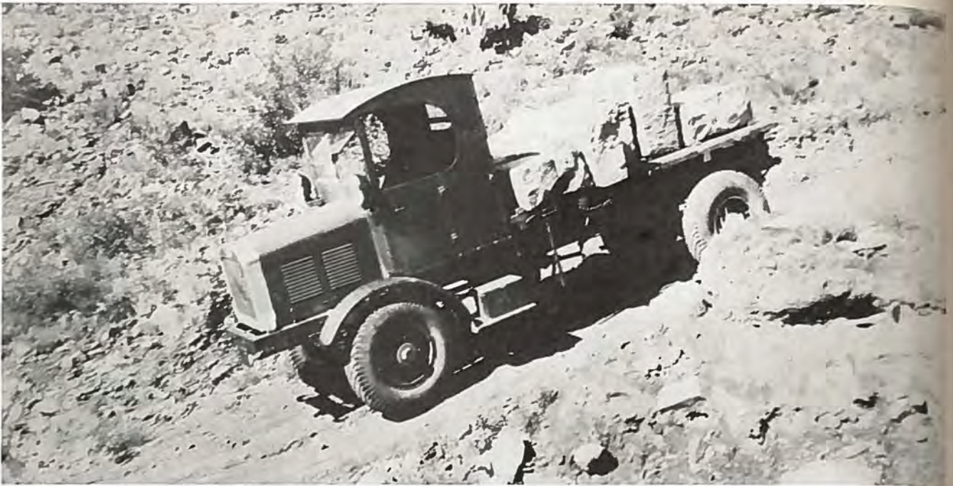
Three and a half-ton F. W. D. CU-6 model coming down an 18% grade. Second gear held the load back without using brakes. James N. Warner, Salida, Colo., owner. FWDs are at work on the highways of the world 12 months per year
