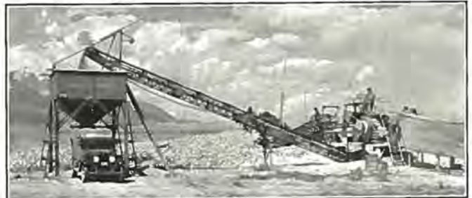
No. 12B Pioneer Screening, Crushing and Loading Plant owned by Threet Bros., Lovell, Wyoming, operating in Teton mountains in Wyoming and producing large daily capacities
