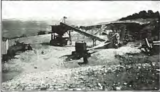
No. 12-B Pioneer Screening, Crushing and Loading Plant and Pioneer Power Unit in operation at Walsenburg, Colorado. This Plant is the property of Mountain States Construction Company, Pueblo, Colorado.
