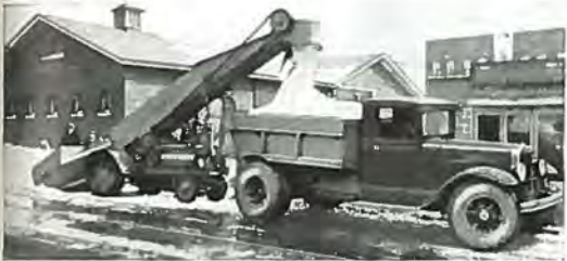
Streets are cleaned fast with this McCormick-Deering-powered snow loader and an International Speed Truck.
