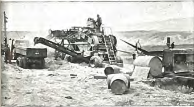
No. 12 Pioneer Screening, Crushing and Loading Plant. Screens, crushes and loads in one operation. Capacity 350 to 500 cubic yards per day, depending upon amount of oversize. The plant pictured here is owned by Fred Redman, contractor of Wenatchee, Wash., and has special equipment of double pneumatics, both front and rear. It also has a special "hookup" consisting of a No. 3 Pioneer Shaker Screen set ahead of plant to remove large amount of fines. A blower may be installed over the auxiliary screen to insure positive rejection of all dust particles and fines.
