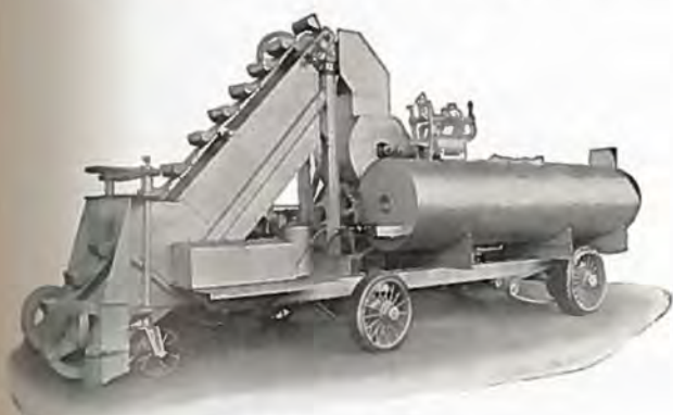
View of Road Mixer Showing Heaters and Bitumen Storage Tank
