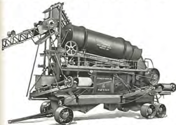
No. 300W Pioneer Washing, Crushing, Screening and Loading Plant produces large daily capacities of washed aggregate, pea gravel and sand. Plant is portable. Send for 3-color detailed circular No. 98, also rotogravure broadside of Pioneer Plant on Stone & Webster Rock Island job.
